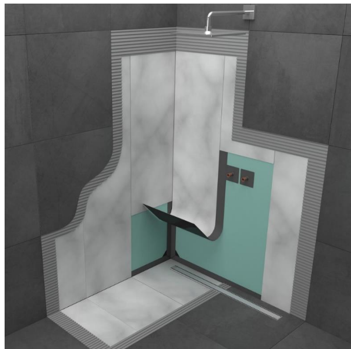
Figure 3: Self-Adhesive Waterproofing in Toilet
